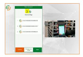
The next screen shows the current Scanning Session which counts and shows the RFID tags that are being scanned. You can now use the device's Trigger to Start scanning.
